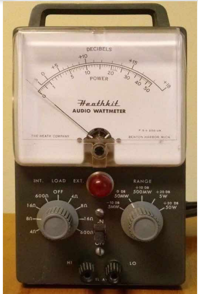
Figure 8: A “Classic I” style AW-1 with a red plastic pilot lamp lens. Possibly a user change? Maybe a Heathkit change to initially replace the red jeweled lamp. (web photo).
