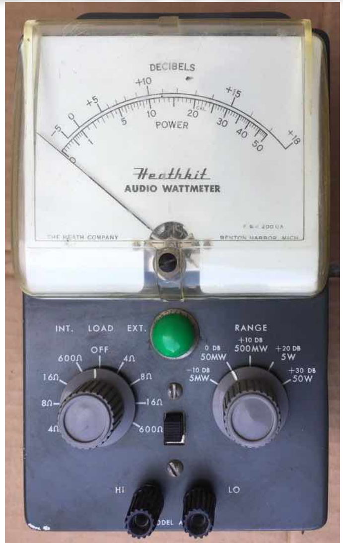
Figure 7: A "Classic I" style AW-1 with later green plastic pilot lamp lens (web photo).
