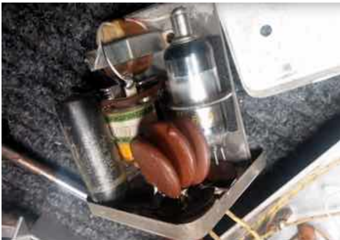
Figure 6: The Victoreen #667 HV unit, with the cover unsoldered, used in the Heathkit RC-1. Note the inductor/transformer, the relay, the foam mounted tube (type unknown), one tubular capacitor and some disc ceramic bypass capacitors.
