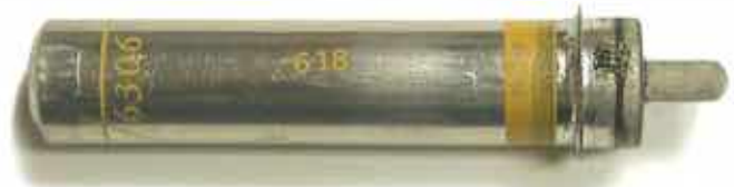
Figure 7: 6306 Geiger Müller tube manufactured by the Victoreen Instrument Company,
