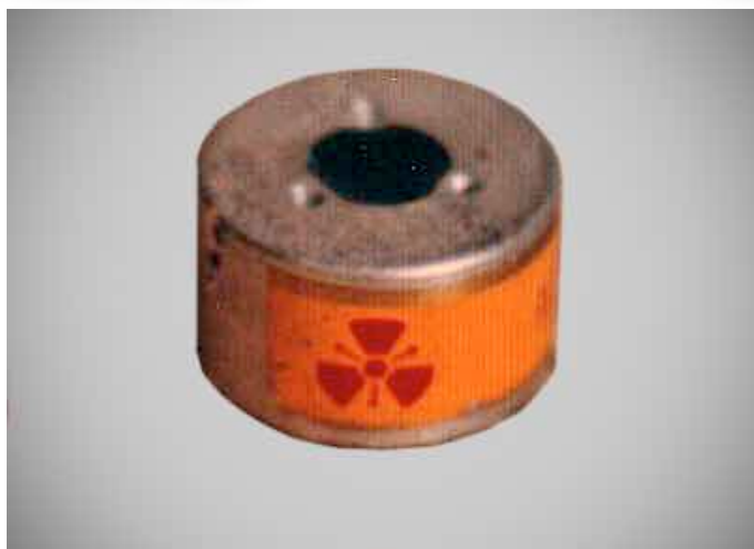
Figure 4: Heathkit PN 419-1 Radioactive Sample used for calibration. It produces 1 mR/hr. Photo courtesy of Chuck Penson - WA7ZZE
