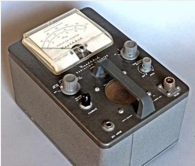
Figure 1: The Heathkit RC-1 Radiation Counter (Geiger Counter) less probe. Photo courtesy of Chuck Penson - WA7ZZE.
