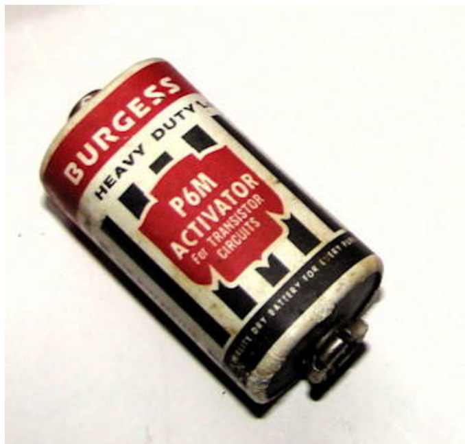
Figure 3: The NEDA 1600D (Burgess P6M) battery believed to be supplied with the early HD-20 kits. A round NEDA 1600 (Burgess P6) fits as well.
