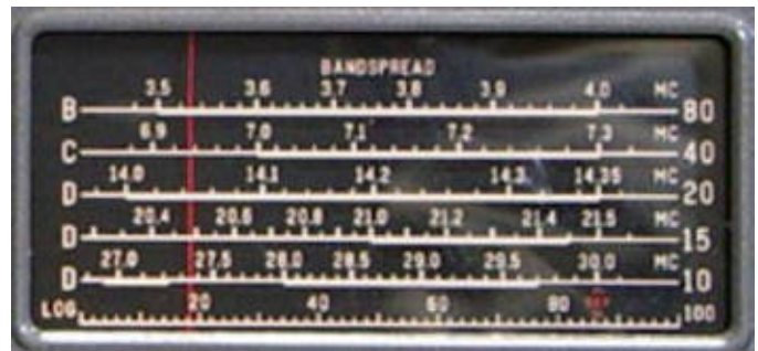
Figure 2: Typical 50's bandspread dial. This one is from a National Radio NC-88 / NC-98.
