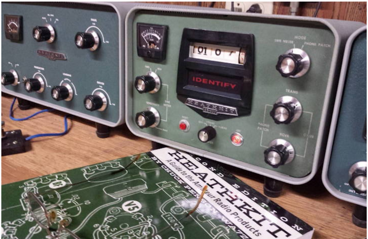
Figure 6: A nicely restored Heathkit SB-630 Station Console sits between an SB-500 2 Meter Transverter and an SB-610 Monitor Scope in the Heathkit shack of WB4IUU. See the restoration at:
