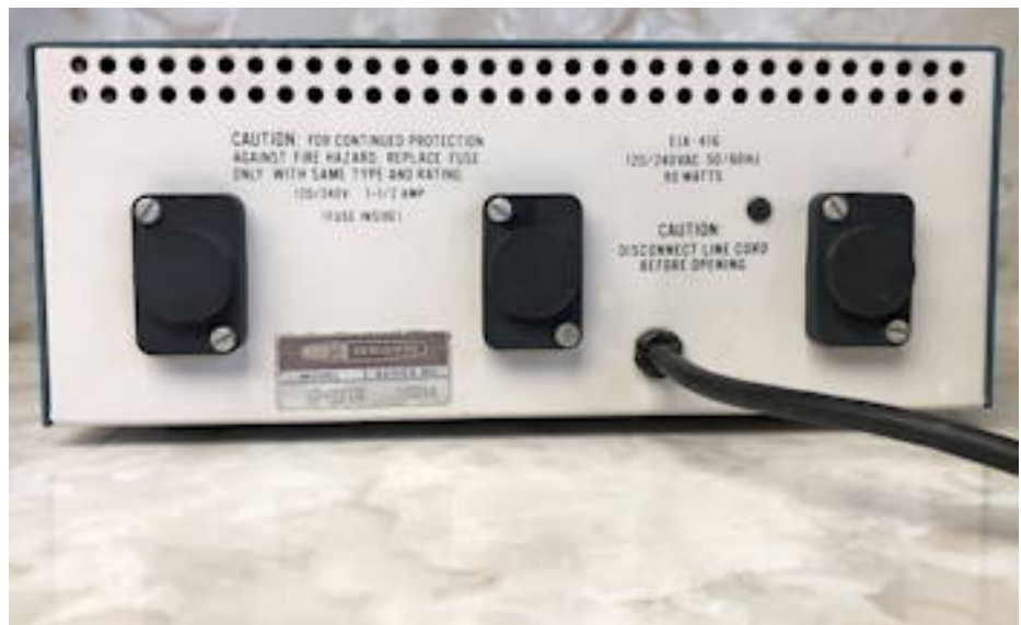
Figure 3: Rear view of the IP-2718 showing line cord and covers for the 5V IC regulator and two MJ2841 power transistors. Photo: AF6C
