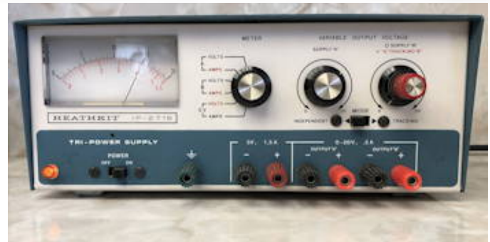
Figure 1: Heathkit IP-2718 Tri-Power Supply with three outputs of 5 V @ 1.5 A fixed, 0 - 20 V @0.5 A and a second 0 - 20 V @0.5 A. Photo: AF6C
