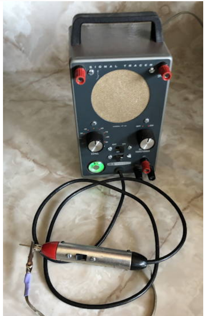
Figure 1: The refurbished IT-12 Showing the probe, bright 1629 eye-tube and later style knobs. The probe features an authentic #477-3 Solder less probe tip replacing the broken one on the unit as received.
