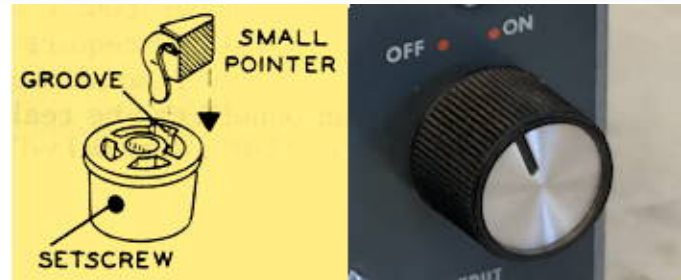
Figure 3: Left: a drawing shows the assembly of the knob (with setscrew in place) #462-139 and pointer #463-27 on early units. Right: Later units had a knob with a painted line #462-187 and no setscrew, which was supplied separately.
