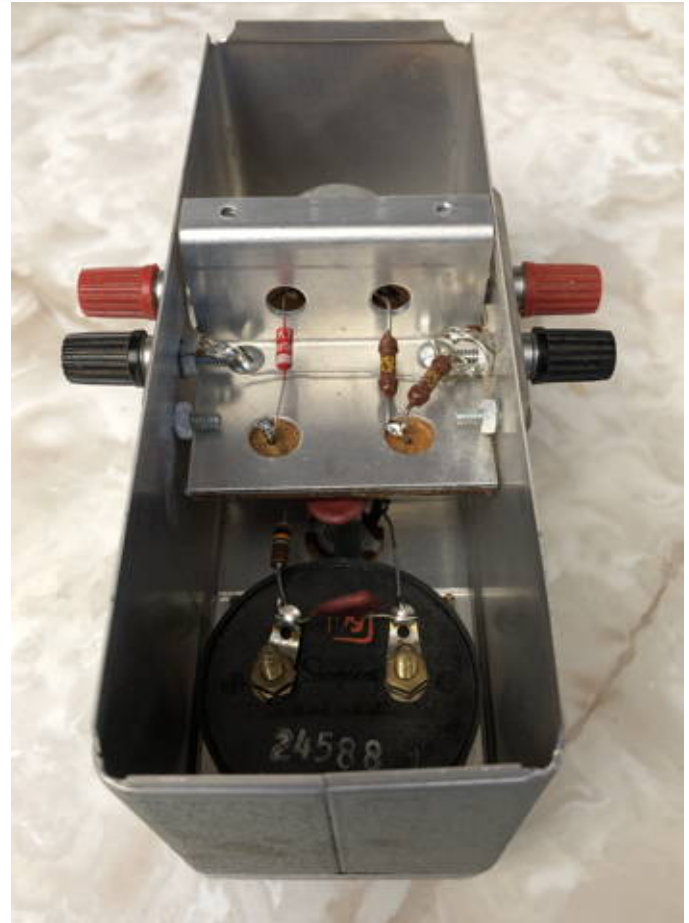
Figure 10: The AM-1 with the rear cover off, looking in with the bottom towards you. The meter is visible lower center with a 0.005 capacitor across its terminals and the 10K resistor off the terminal to the left. Above the chassis are the diode (left) and the two precision resistors (right). Just visible sticking out below the chassis (center) is the other 0.005 capacitor.
