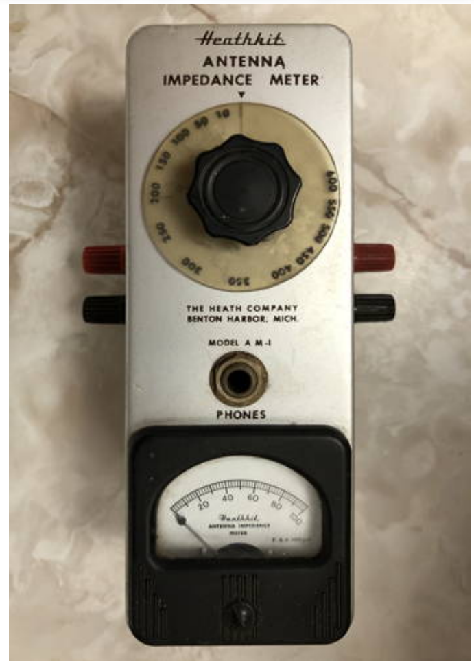
Figure 1: The Heathkit AM-1 Antenna Impedance Meter. The fifth Heathkit amateur product.
