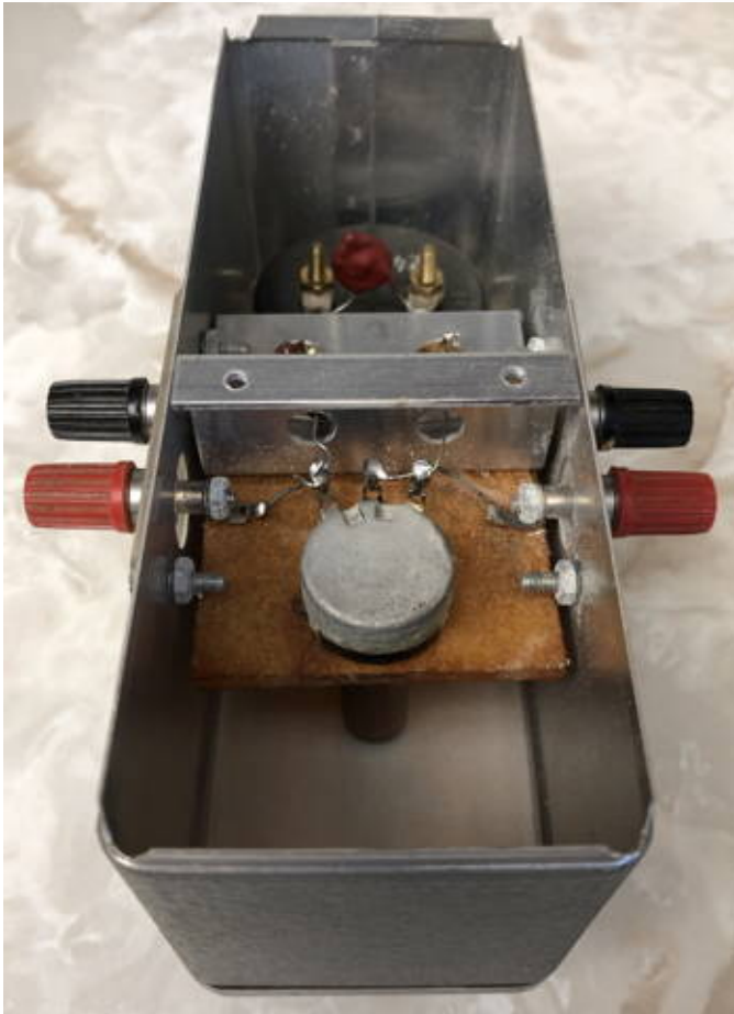
Figure 9: The AM-1 with the rear cover off, looking in with the top towards you. Note the two red binding posts. The back of the control is mounted on the insulated plate with the insulated shaft extending through the front panel for isolation.
