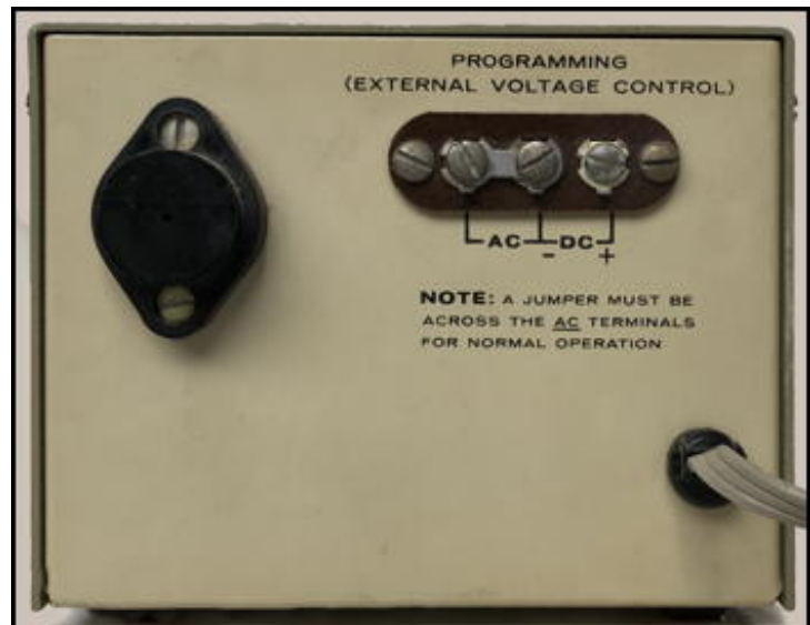
FIGURE 12: A view of the rear of the IP-18 showing the programming terminal strip. Insulated transistor is on the left and the power cord exit is on the right.
