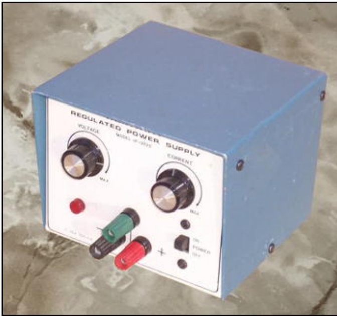
Figure 3: The newly styled Heathkit IP-2728 that replaced the IP-18 in 1977.
