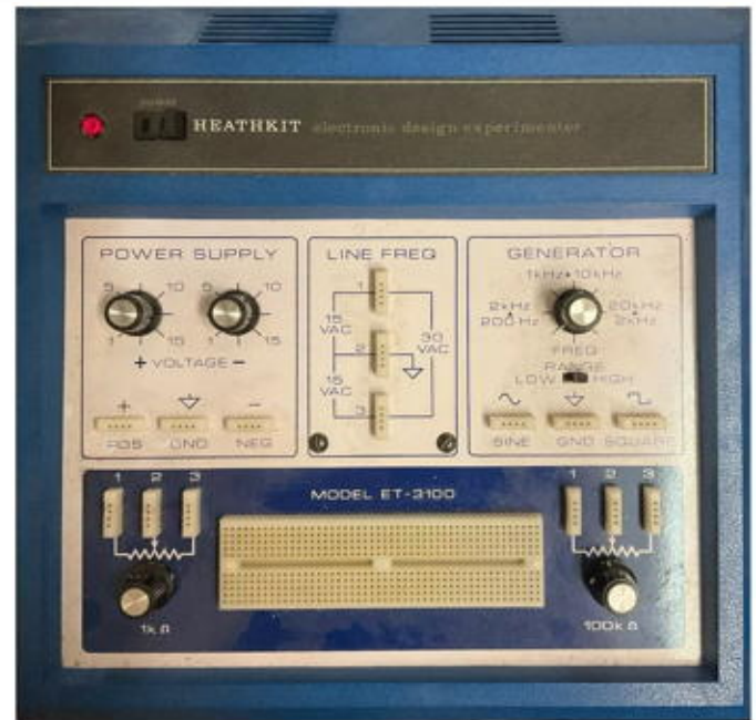
Figure 1: Original ET-3100 Electronic Design Experimenter (Trainer) showing the two power supply controls, the 15/30 VAC line frequency terminals, the generator controls, the two undedicated potentiometer controls and the breadboard area.
