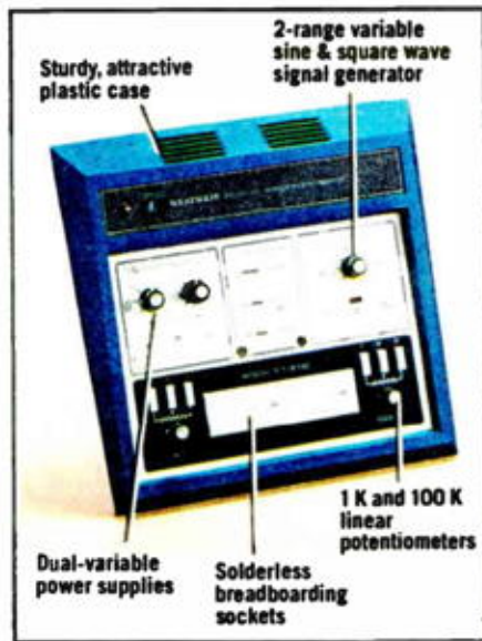
Figure 3: The ET-3100A Ad from the December 1981 catalog. Note the ' 1.2 to 16 volts, current rating 120 mA ' specifications. See text for details. Note also that a Spanish language Manual was available.
