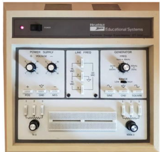
Figure 5: The ET-3100B, showing a white color style silkscreened on the circuit board (85-2730-3) that makes up the front panel.
