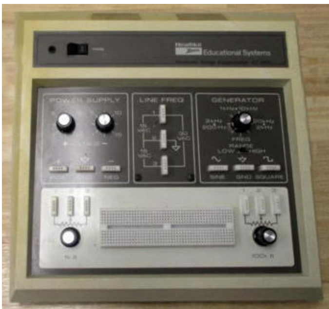
Figure 4: The ET-3100B, showing a brown color style silkscreened on the circuit board (85-2730-1) that makes up the front panel.
