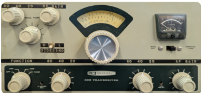
FIGURE 14: is a photograph of Pete's THW-32 that he purchased off eBay, after he cleaned it up considerably. Originally an HW-32, it has been converted to a tri-band radio. Pete is looking for the THW-32 conversion manual that came with the kit.
