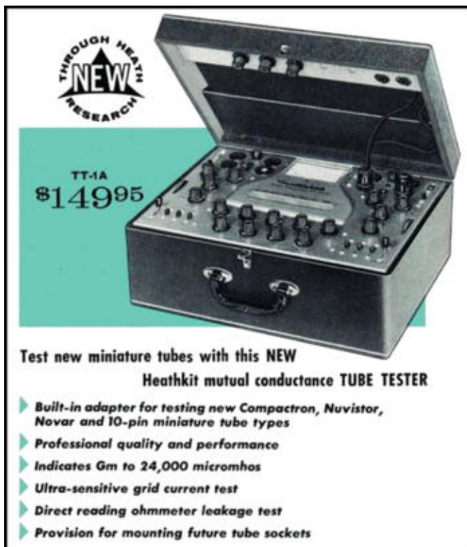
Figure 6: The TT-1A Mutual Conductance Tube Tester. (March 1962 Catalog - page 30)
