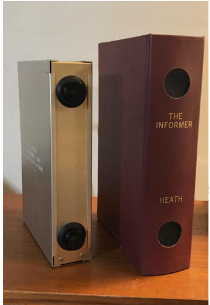
Figure 1: The Heathkit GD-39 book-like Intrusion Alarm. On the left is the unit; on the right is the book-like sleeve it slides into for concealment.
