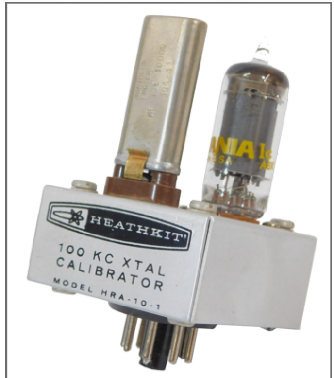
Figure 1: The Heathkit HRA-10-1 Crystal calibrator that may be plugged into the HR-10(B) receiver or one of the Single-Bander transceivers.
