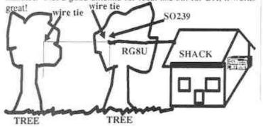
Antenna is not affected by plants or other non-metallic objects. Also the half wave does not have to be perfectly straight to work properly.
