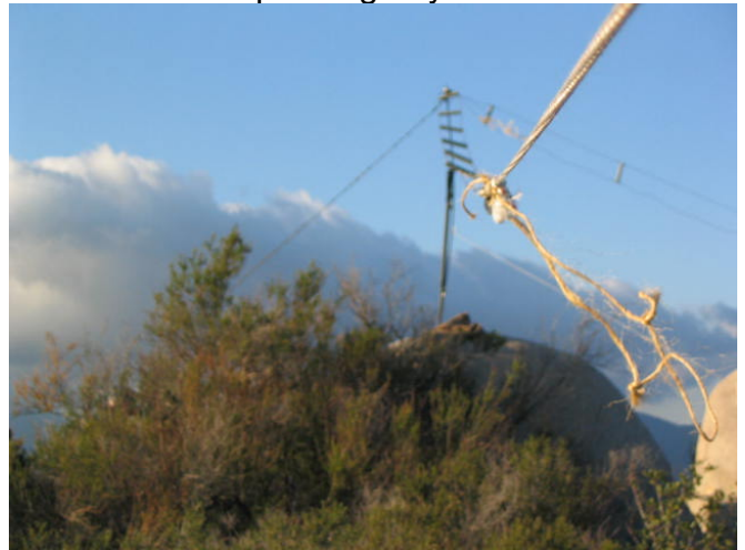
20M/40M antenna with 450Ω Ladder line Feed
