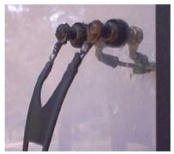
Figure 2 - Window feedthroughs.
