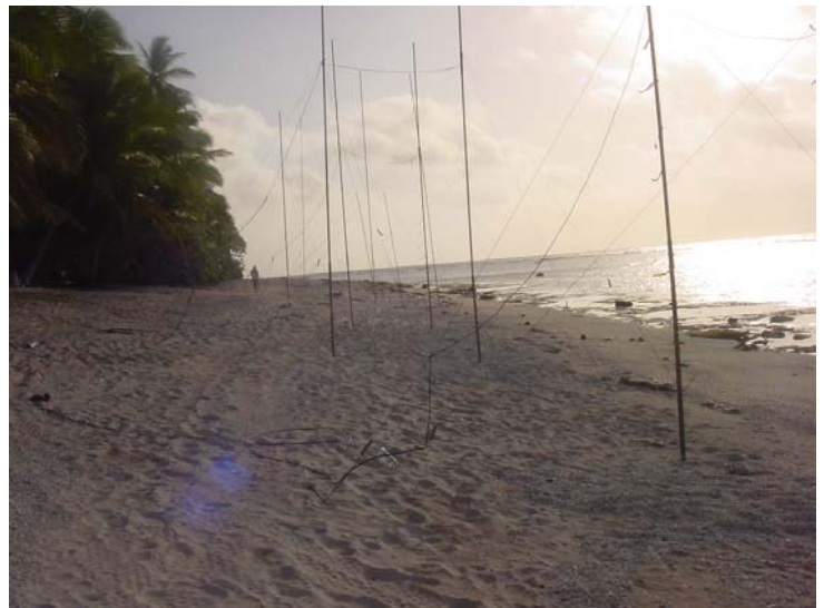
The beach made a perfect location for a vertical “Antenna Alley” with plenty of sand and salt water for the radials.
