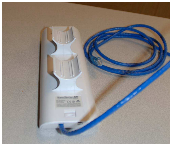
Fig02 – A Hamnet “Nano Station” from Ubiquiti contains two access points
