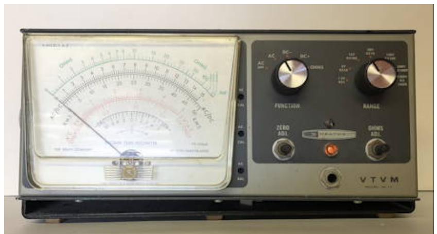
Figure 5: Heathkit IM-13 Deluxe "Service Bench" VTVM In the Classic II style, and in the new horizontal format. Note calibration access holes to the right of the meter. Photo by author.
