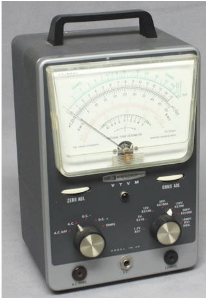
Figure 4: Heathkit IM-32 Deluxe "Service Bench" VTVM The Classic II style update of the IM-10. It was the last of the vertically oriented Bench VTVM. Photo courtesy of Sonny Clutter, www.radiolaguy.com .
