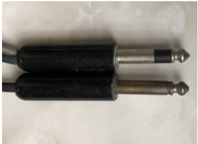
Figure 6: Top shows the new phone plug with its thicker insulation to prevent flashover at higher voltages. Below it is the standard phone plug used on the earlier VTVMs.
