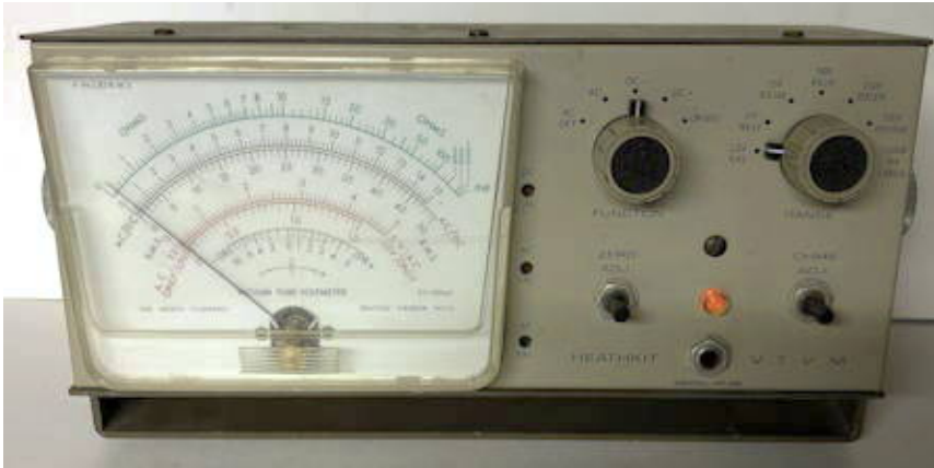
Figure 7: Heathkit IM-28 Deluxe "Service Bench" VTVM In the "New Look" style. It is the first of the series to use a 120/240 V primary transformer and a three-wire AC plug. Photo by author.
