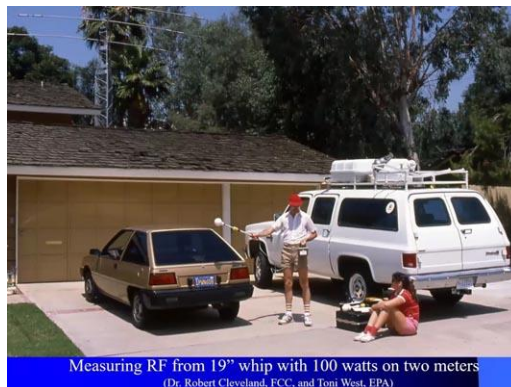
Fig 10 – Measuring RF from a 19" whip with 100 watts on two meters
