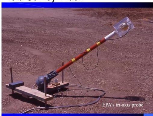
Figs 8 and 9 – Measuring the RF field near a rover running 1 kW
