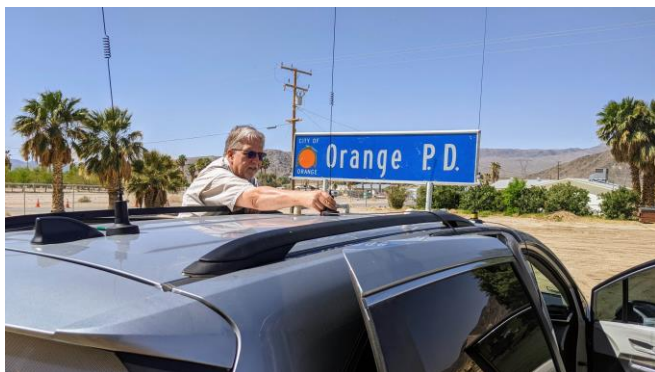
Fig03 - Jeff KK6YUP installs the Ham antennas on the Follow-Vehicle at Baker HS before the race. In addition to the APRS beacon on 2M, there are two more radios for 2M voice and 440 voice com. The OPD drivers are required to also provide FRS radios. The FV provides location, condition of runner, water, and food for the runner.
