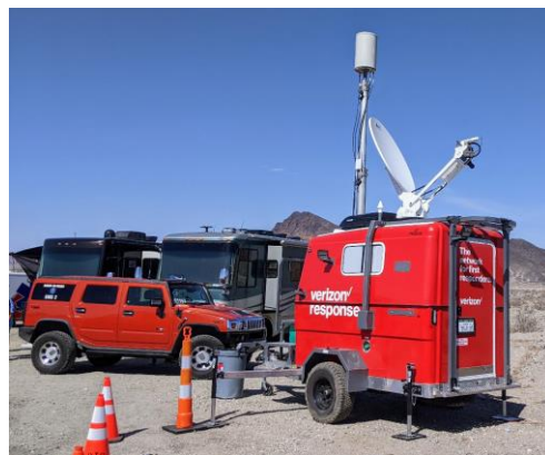
Fig17 – Technology is CHANGING!!! The B2V desert used to be a “desert for cell-phone coverage”. This year, Verizon provided enough mobile Cell-Phone towers with satellite dishes (for the “back-haul”) to provide coverage at every race-checkpoint. Using these Verizon towers...the OPD team captains in Las Vegas could obtain official running times over the internet from the runner-batons, before the Follow Vehicle could report the leg-running-time to LV by ham Radio.
