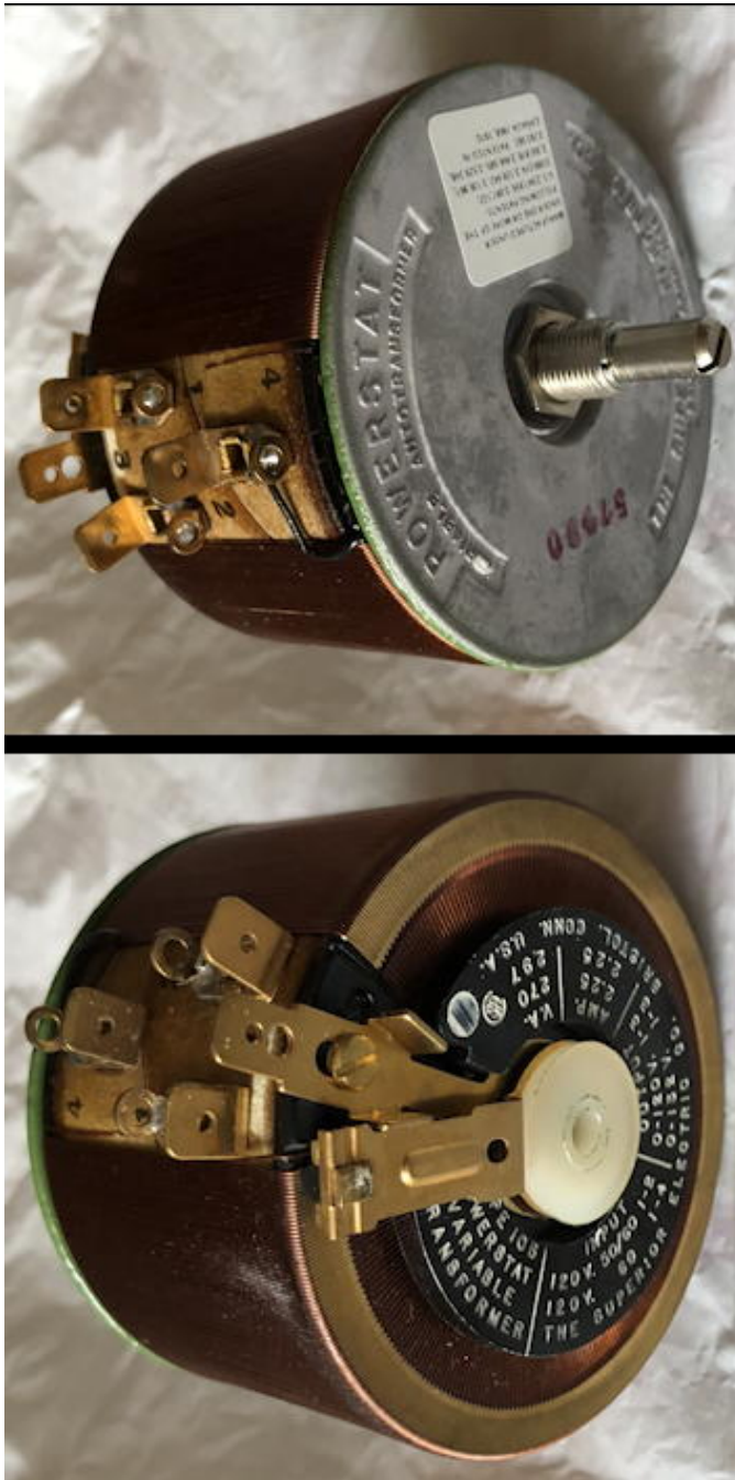
Figure 4: A variable autotransformer similar to T1 that is used in the IP-5220. This is a Powerstat 10B made by the Superior Electric Company.
