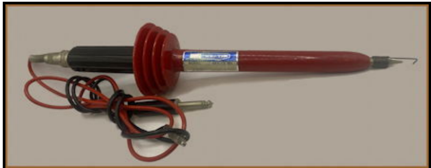
Figure 8: #336 30 kV HV Probe. This probe mounts in a red and black plastic body that Heathkit used for all their HV Probes (Part # 476-2) with the exception of the early #310.
