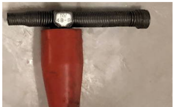
Figure 3: The Spring adapter P# 432-197 that comes with the Heathkit CI-1020 is designed to mate between the spark plug wire and either the spark plug or distributor cap terminal.
