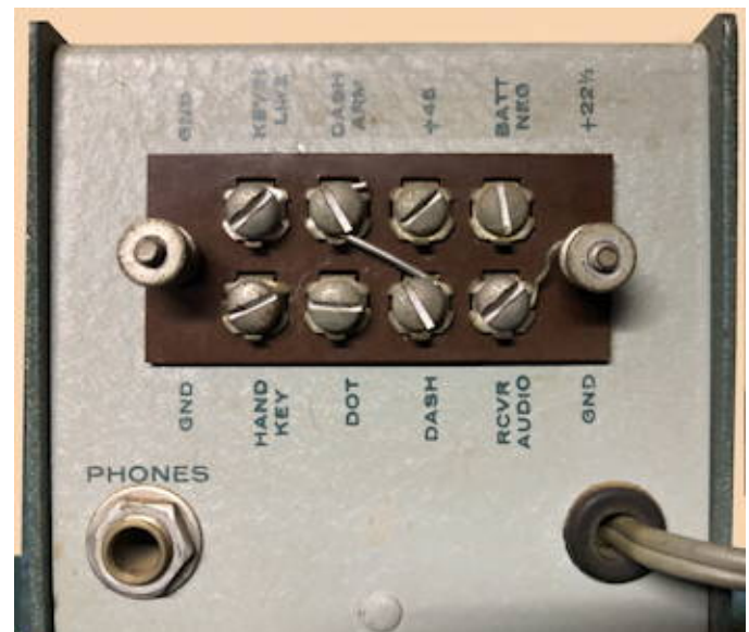
Figure 2: Rear panel of the HD-10 Keyer showing the eight screw terminal strip. The two thumb-nuts on the mounting studs are grounds. Also shown are the phones jack and line cord exit.
