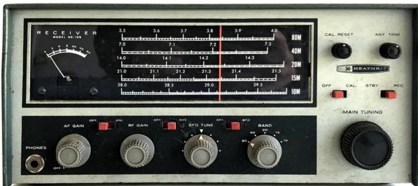
Figure 4: A larger view of the HR-10B front panel. Note that the 15 meter scale goes to 21.50 MHz though the band ends at 21.45. The AM/SSB frequencies are marked by a thickened white bottom line.
