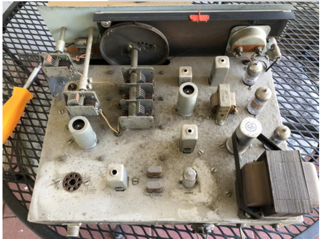
Figure 9: Removing the cabinet revealed a lot of dust that needed to be removed. The reason for the tape around the filter capacitor and transformer is, as yet, unknown.
