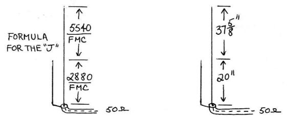
Results of tests on single "J" Antenna compared with a quarter-wave vertical test freq. was 145.54 MHz. Both vertical and "J" were mounted at same height, ten feet at the tip.
