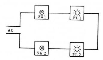
Switch (SW1) controls only light (PL1) and switch (SW2) controls only light (PL2). What is the circuit in each black box?
